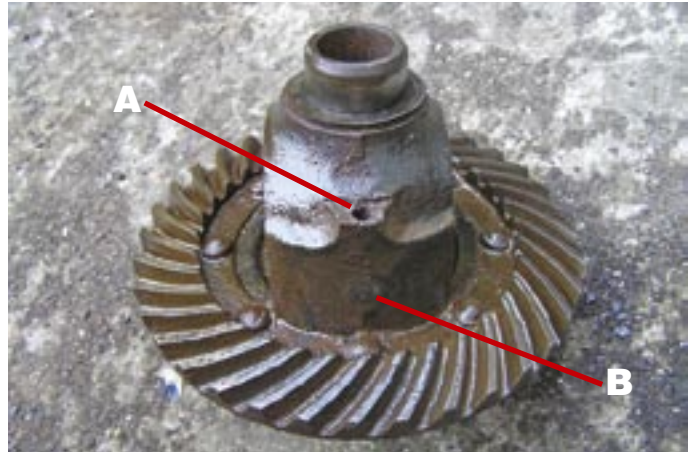
Remove the lock pin (A) and then press out the differential pin (B). The eight rivets around the crown wheel need to be faced off and drilled out.
