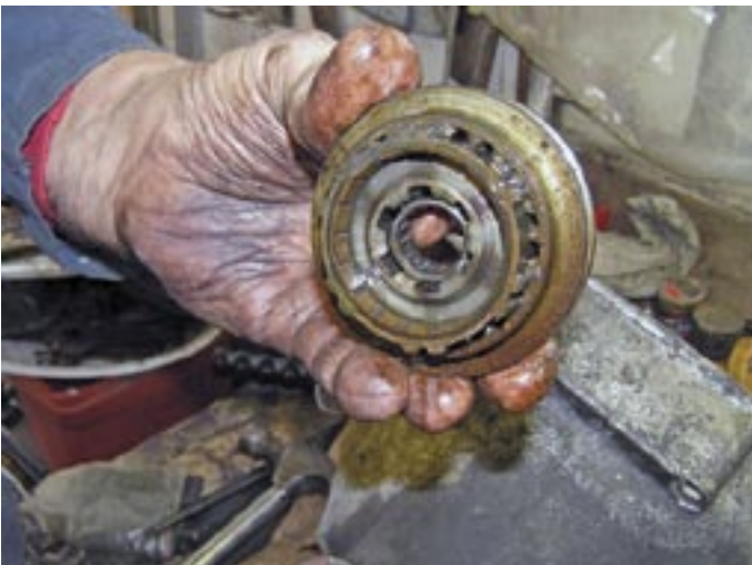
... making sure that the centre bearings are not damaged.
