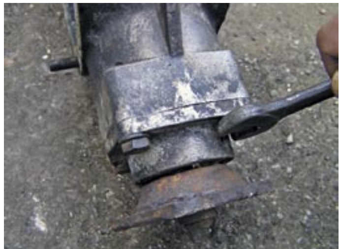
Unbolt the four bolts around the coupling flange to release the pinion assembly from the axle housing.
