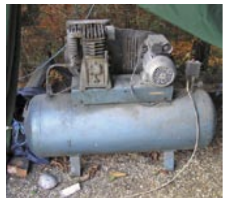
If using an air compressor, use a powerful one, and fit a water/oil trap on the pipeline.
