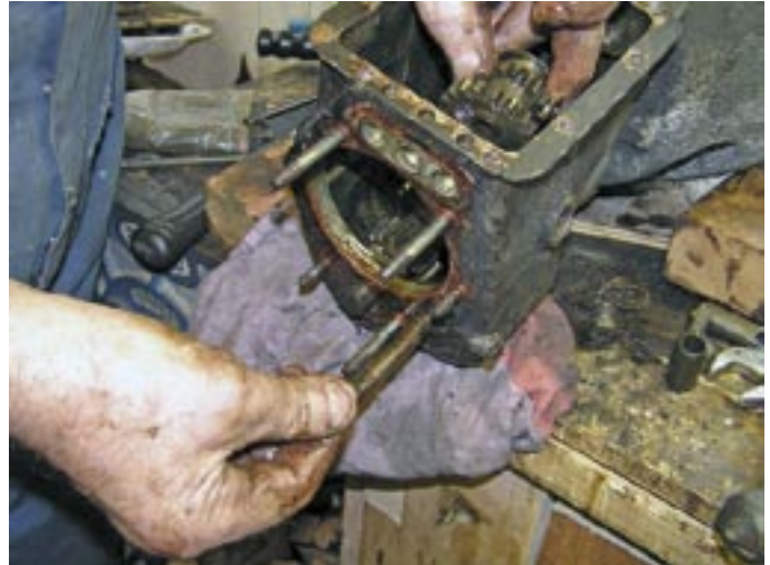
Remove the reverse gear lockpin, tap out the reverse shaft, and lift out the reverse gear assembly.
