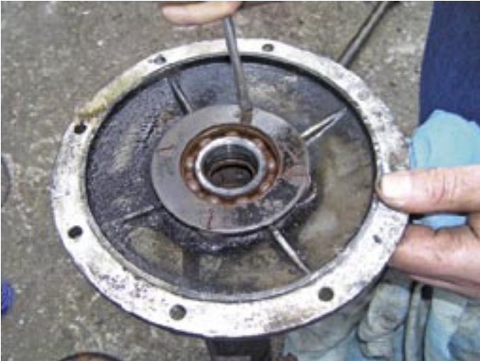
The differential bearings are held behind a retaining plate. Removing the four screws will give access to the bearings.
