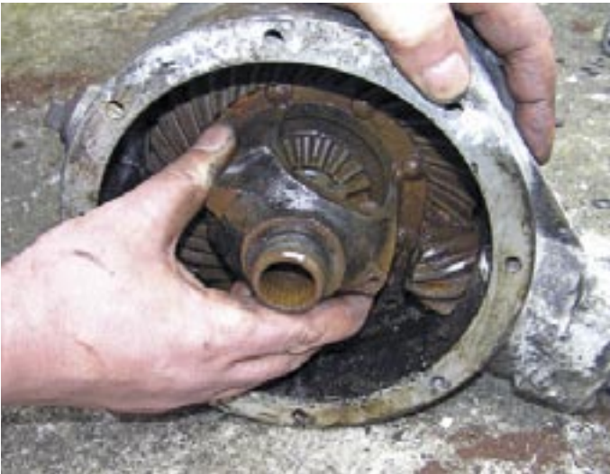
The rust inside this axle is a result of the oil level never being checked.
