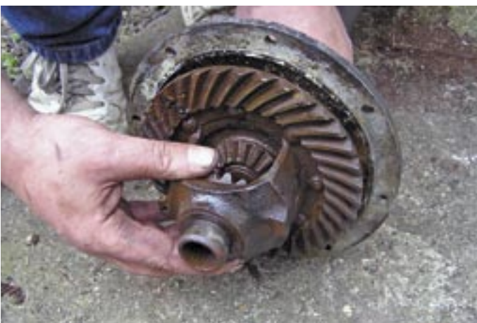
With the outer casing removed you can see the position of the differential case, pinion and crown wheel. This is perhaps ...
