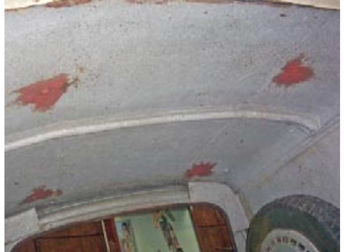
If a roof rack is fitted, ensure there are no leaks inside.
