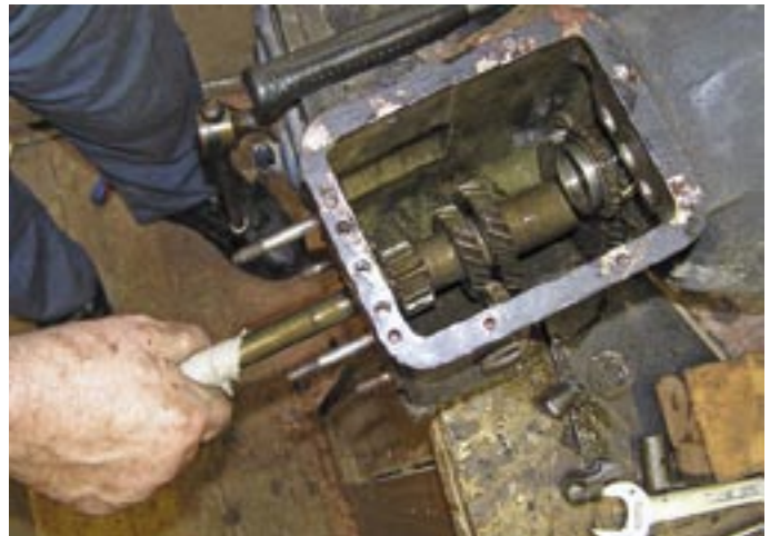
The laygear shaft can be withdrawn along with the main shaft assembly that goes through into the bell housing.
