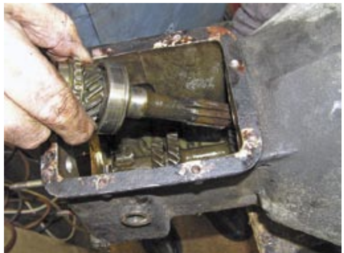
Lift out the main shaft.
