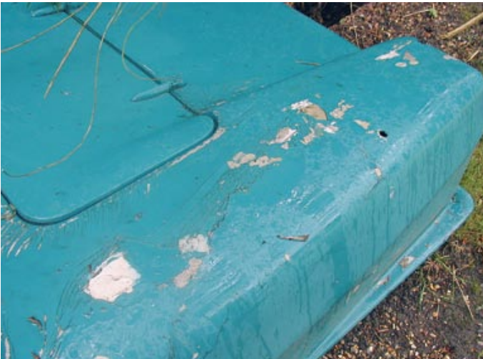
From the same vehicle as shown above, you can see a number of cracks along the wing and patchy repairs. Chances are that damage like this is going to involve a lot of work to put things right.
