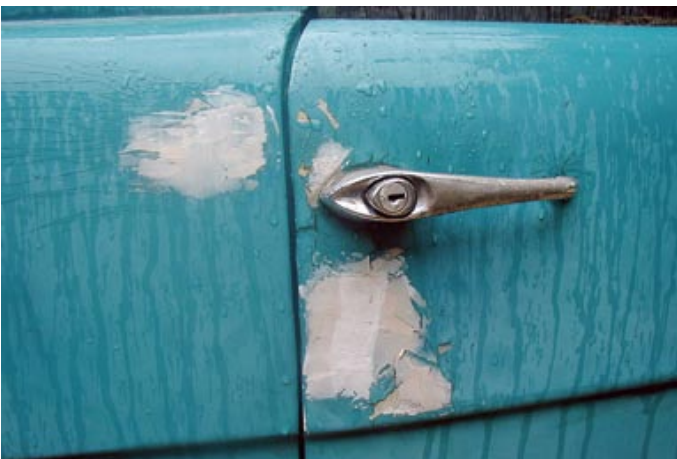
Watch out also for damage around the door handle, as this could weaken the handle mounting points.
